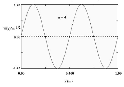
**1.52** When n = 4, three nodes are seen (marked with  $a \bullet$ ):
